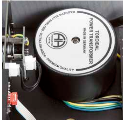
An encapsulated toroidal transformer feeds the Preamp III. It is located at the front left of the cabinet and thus far away from the sensitive inputs.
