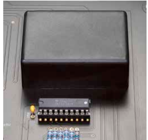
This small black box contains the highly precise volume control, which, like the entire Preamp III, is fully balanced.
