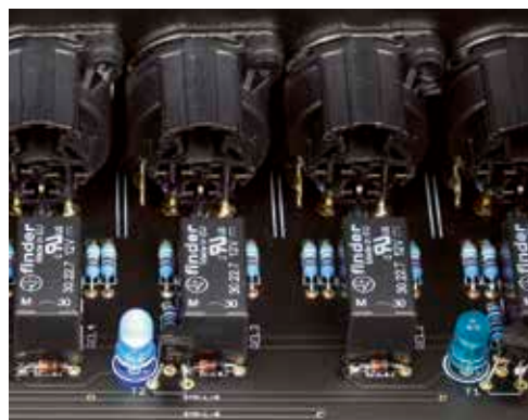
The inputs are switched via extremely tight relays. The assigned blue LEDs can be seen glowing through the top of the housing.
