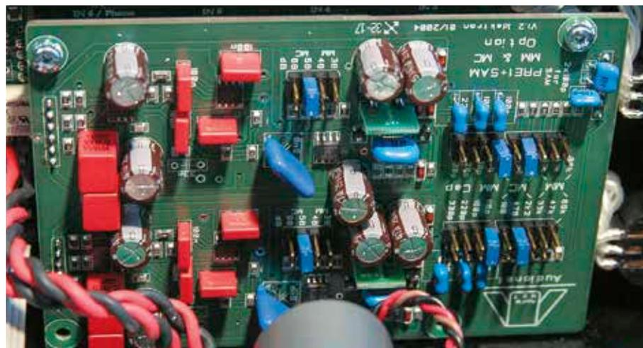
▲ The factory-fit phono section has been reworked for the 20 SE, differing in many details from the 500 Euro optional board retrofittable to the SAM.
